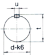
Pump shaft end
